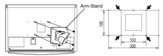
4 Mounting Screws (enclosed): M4 x 12 mm
